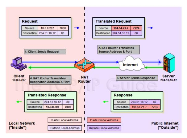
The TCP/IP Guide - IP NAT Port-Based ("Overloaded") Operation: Network Address Port Translation (NAPT) / Port Address Translation (PAT)
